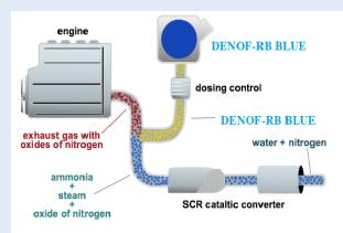
DENOF-RB BLUE is not a fuel or fuel additive. It has it's own tank shown as below. It works as part of SCR (Selective Catalyst Reduction)) system.
